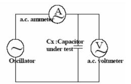
Circuit for leakage current method
