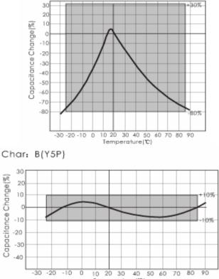
Temperature (°C) Y2 AC Ceramic Capacitor 250VAC
