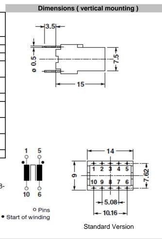
The case are of flame-retardent plastic material in accordance with UL  $94\mbox{V-}0$
