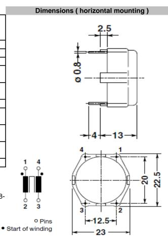
The case are of flame-retardent plastic material in accordance with UL  $94 \ensuremath{\text{V-0}}$
