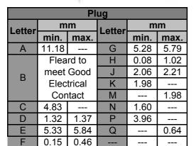
**Note:** I.D. to meet VSWR and contact resistance when mated with 1.32 / 1.37 mm Dia. Pin.
