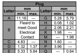
**Note:** I.D. to meet VSWR and contact resistance when mated with 1.32 / 1.37 mm Dia. Pin.
