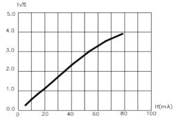
Relative Luminous Intensity vs. Forward Current
