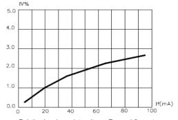
Relative Luminous Intensity vs. Forward Current
