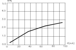
Relative Luminous Intensity vs. Forward Current
