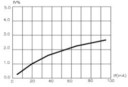
Relative Luminous Intensity vs. Forward Current
