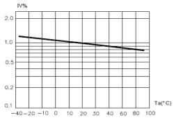
Relative Luminous Intensity vs. Ambient Temperature
