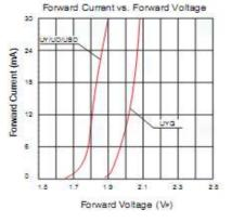
Forward Current vs. Forward Voltage
