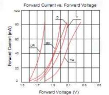
Forward Current vs. Forward Voltage
