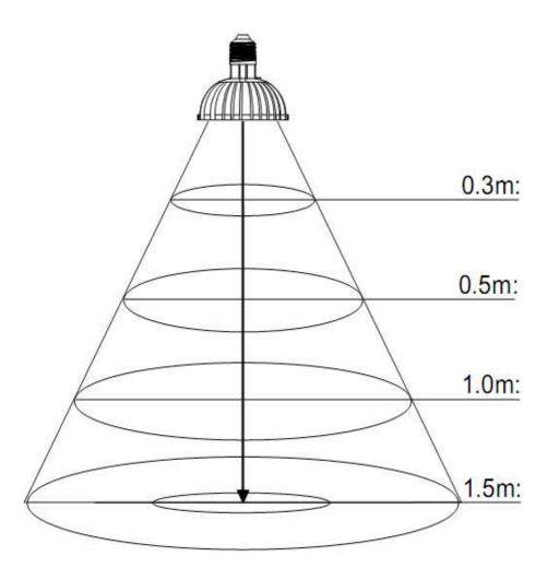
The center beam lux is measured with digital Lux Meter (Model TES-1334-A)
