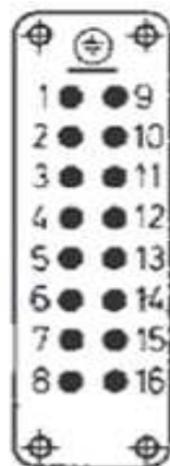
Contacts arrangement view from termination side
