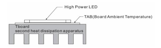
Board Ambient Temperature Tolerance 5℃
