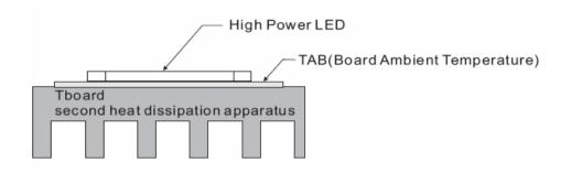
Board Ambient Temperature Tolerance 5℃
