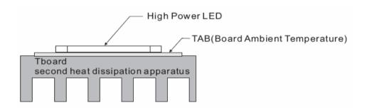
Board Ambient Temperature Tolerance 5℃ TAB in this table is according to highest operating temperature 65℃ The TAB is the stable testing value for the product lighted 100% after one hour Different materials of second heat dissipation device, the surface area of heat sink will be different, Thus, this document is for reference only.
