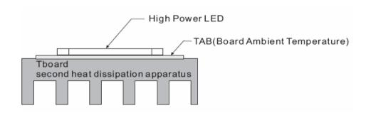
Board Ambient Temperature Tolerance 5℃ TAB in this table is according to highest operating temperature 65℃
