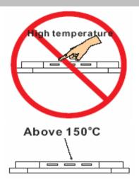
There is 150°C directly from the front of Power LED emitting diode. It is untouchable to prevent burning.
