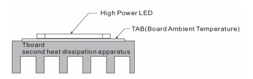
Board Ambient Temperature Tolerance 5℃
