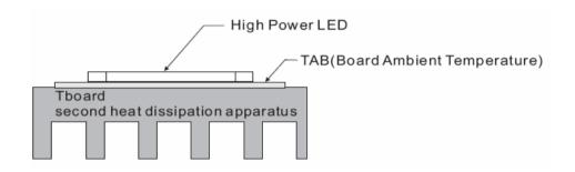
Board Ambient Temperature Tolerance 5℃
