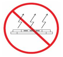
The product should not be light up directly without heat dissipation device
