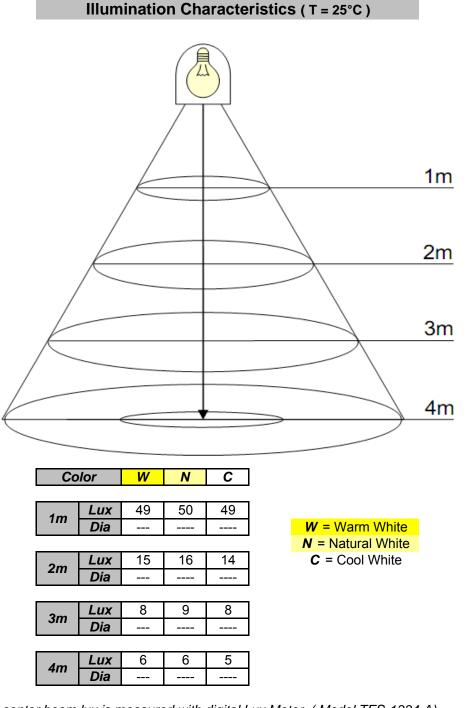
The center beam lux is measured with digital Lux Meter (Model TES-1334-A)
