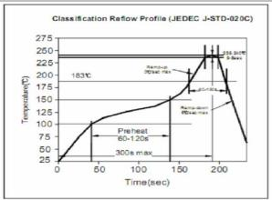
Soldering Profile for Lead Free Soldering 255-260°C
