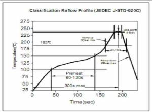
Soldering Profile for Lead Free Soldering 255-260°C
