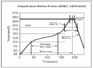
Soldering Profile for Lead Free Soldering 255-260°C
