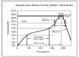
Soldering Profile for Lead Free Soldering 255-260°C
