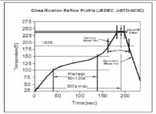
Soldering Profile for Lead Free Soldering 255-260°C
