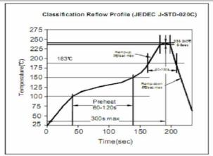
Soldering Profile for Lead Free Soldering 255-260°C
