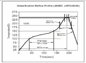
Soldering Profile for Lead Free Soldering 255-260°C
