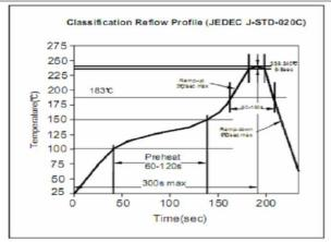
Soldering Profile for Lead Free Soldering 255-260°C
