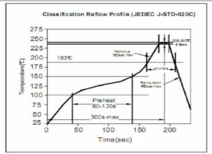
Soldering Profile for Lead Free Soldering 255-260°C
