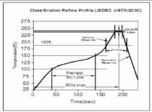
Soldering Profile for Lead Free Soldering 255-260°C
