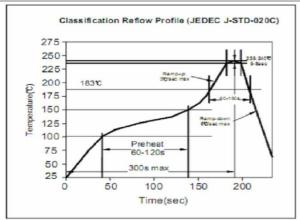
Soldering Profile for Lead Free Soldering 255-260°C
