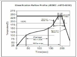
Soldering Profile for Lead Free Soldering 255-260°C
