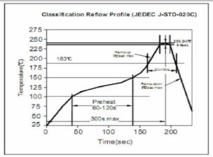
Soldering Profile for Lead Free Soldering 255-260°C
