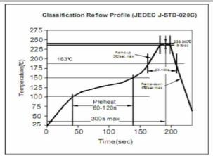
Soldering Profile for Lead Free Soldering 255-260°C
