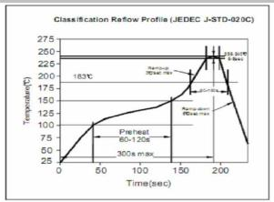
Soldering Profile for Lead Free Soldering 255-260°C
