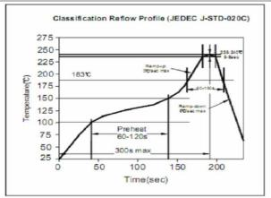
Soldering Profile for Lead Free Soldering 255-260°C
