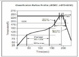
Soldering Profile for Lead Free Soldering 255-260°C
