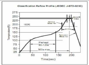
Soldering Profile for Lead Free Soldering 255-260°C
