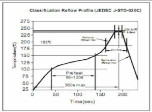
Soldering Profile for Lead Free Soldering 255-260°C
