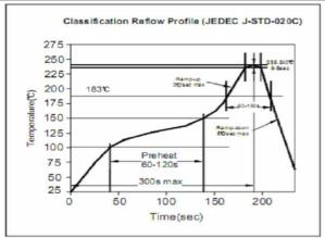
Soldering Profile for Lead Free Soldering 255-260°C
