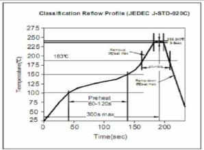
Soldering Profile for Lead Free Soldering 255-260°C
