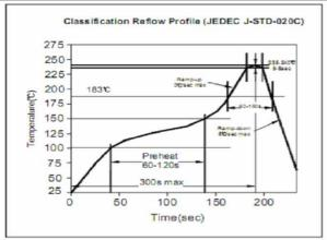
Soldering Profile for Lead Free Soldering 255-260°C
