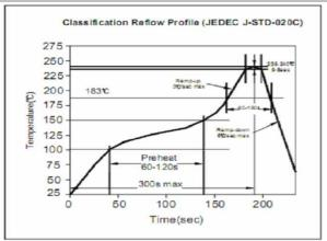
Soldering Profile for Lead Free Soldering 255-260°C
