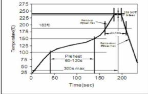
Soldering Profile for Lead Free Soldering 255-260°C
