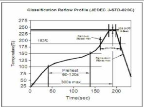
Soldering Profile for Lead Free Soldering 255-260°C
