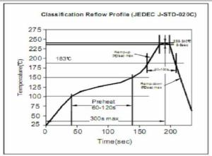
Soldering Profile for Lead Free Soldering 255-260°C
