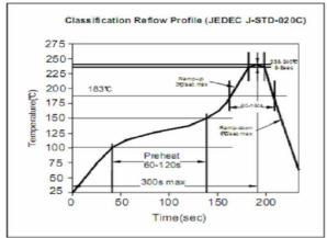
Soldering Profile for Lead Free Soldering 255-260°C
