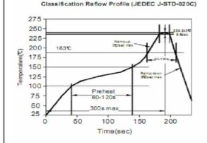
Soldering Profile for Lead Free Soldering 255-260°C
